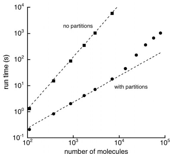
Systems with more than 10,000 molecules simulated less efficiently than smaller ones. Based on code profiling results and cross-platform comparisons, we found that this arises from computer hardware constraints: the smaller simulations kept most data in cache memory, whereas the larger ones used the slower main memory.
